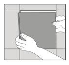
Use a recommended contact adhesive to glue the new tile into place. Follow the installation instructions on its label.
