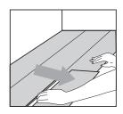
The released plank can then be pulled out.
