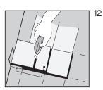
The last and first plank can be cut in the correct width. Place the last plank on top the second to last plank.
