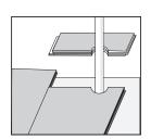
Drill the required holes in the planks, making a hole on the plank 10mm (3/8") bigger than the pipe diameter.
