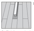
Cut off the locking groove rebound on the short and long sides of the new plank.
